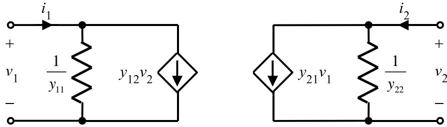
Short-circuit admittance parameters are useful for combining two two-port networks that are connected together in a **Parallel-Parallel** configuration. The admittance parameters conveniently add together, as shown below:
