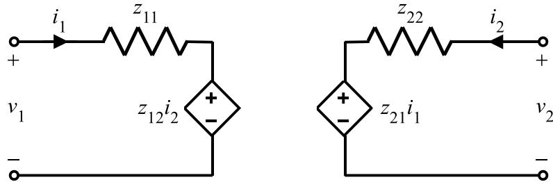
Open-circuit impedance parameters are useful for combining two two-port networks that are connected together in a **Series-Series** configuration. The impedance parameters conveniently add together, as shown below:
