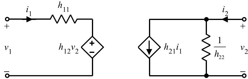
Hybrid parameters are useful for combining two two-port networks that are connected together in a **Series-Parallel** configuration. The hybrid parameters conveniently add together, as shown below:
