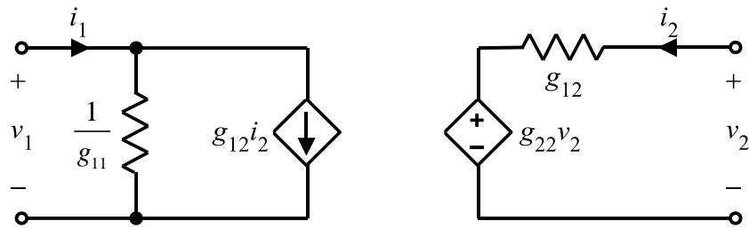
Inverse hybrid parameters are useful for combining two two-port networks that are connected together in a **Parallel-Series** configuration. The inverse hybrid parameters conveniently add together, as shown below:
